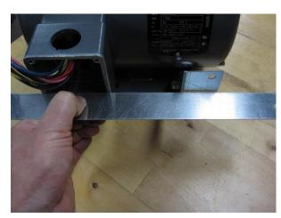
**4b. 7.5 & 10 HP Idler/floor Bracket (7.5 & 10HP)**Align and tighten the bracket to the idler flange as shown, leaving approximately a 1/16 inch gap from the plane of the idler conduit box face. Apply the double side tape to the face of the bracket to that it will seat flat to the back of the enclosure. (enclosure removed for clarity)
