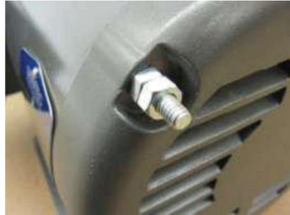
When installing brackets on Rotary Phase Converters 5HP - 15 HP, four extra nuts are provided. These bolts need to be installed as shown here to protect the idler from the brackets.
