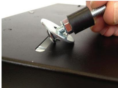
Slide each mounting bolt to approximate position in each slot. Loosely tighten lock nut and rubber isolation mount so adjustments can be made.
