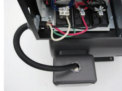
The supplied idler cable has ring lugs at one end, which go to the idler. The other end goes to the panel. Refer to main installation manual when making these connections.
