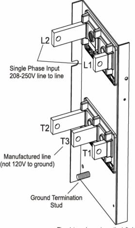
The picture above shows the left side of the converter as installed. The right side is a mirror image. Both sides are live and can be used
