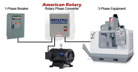
An additional 3-phase breaker panel may be installed on the line between the converter control panel and the 3-phase equipment. This is recommended to protect each piece of equipment and the wire that feeds that equipment.
