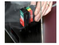
(clear cover used for clarity) Firmly snap in the green, yellow & red switch terminals into the pushbutton switch body.
