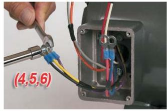
**7.** Bolt motor leads (4,5,6) together. Insulate this connection with electrical tape or heat shrink tubing.
