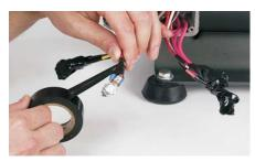
**6.** Terminate motor side wiring with ring lugs that take a 1/4 inch bolt. Bolt these wires to motor lead pairs (1,7) (2,8) (3,9). Insulate connections.
