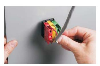
**9.** Snap the red yellow and green switch terminals into the switch receptical on the back side of the cover. Red on the left with the cover hanging upside down as in #8.
