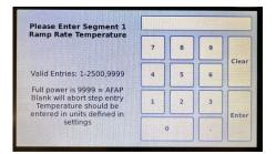
Enter ramp rate in degrees per hour. For maximum rate enter 9999
